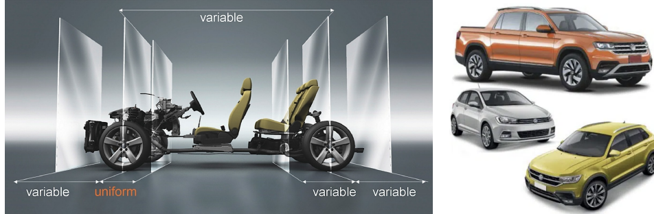
Figure 1: Modular design rules (left) and compatible products (right) at Volkswagen
